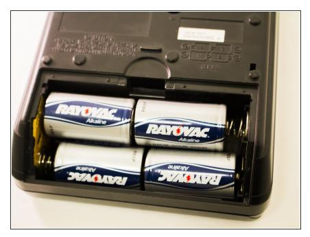
Open the battery compartment by pressing down on the small tab along the upper edge of battery cover.
