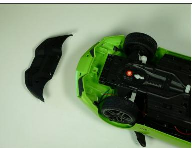
Unscrew the two 2.5 mm Phillips #00 screws from the underside of the car and remove the front underskirt.
