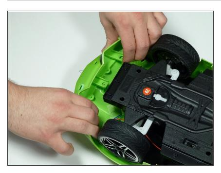
Remove the front bumper by sliding it away from the car.
