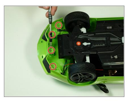
Unscrew the four 2.5mm Phillips #00 screws from the front bumper and lift up the front bumper to remove.
