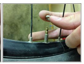
Use you thumb and index finger to unscrew the valve nut by rotating it counterclockwise.
