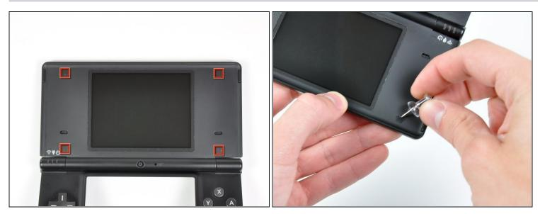
• Use a pushpin to remove the four plastic screw covers (highlighted in red) on the front bezel.
