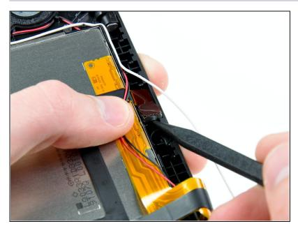
Pry the front-facing camera straight up out of its housing in the front bezel.
