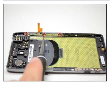
Remove the three 3.5mm Torx T3 screws holding the power/volume button cable to the side of the frame.
