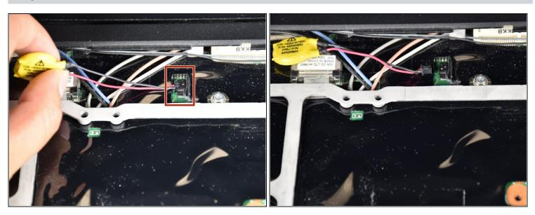
• Pull on the black connection piece and remove the back-up battery.
