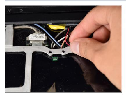
• Gently pull the back-up battery from underneath the front panel.
