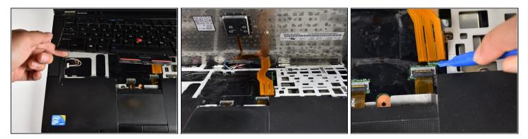
• Lift up the keyboard, but be careful not to completely remove.
