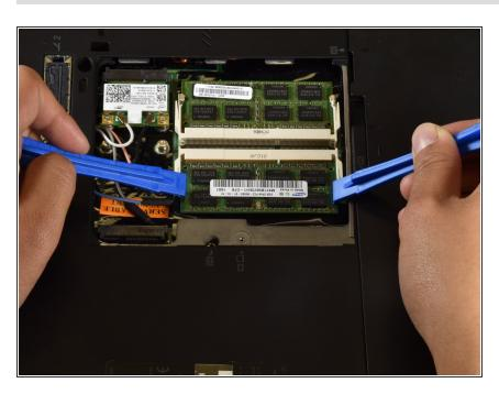
Use two plastic opening tools to lightly pull the two semi-circle tabs apart.
