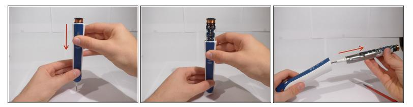
• Push the point of the device down onto the table and take out the inside.
