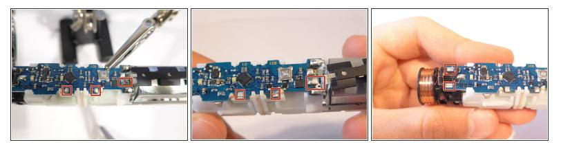
Now you have to desolder the sensor connection and both the connections to the red led at the top.
