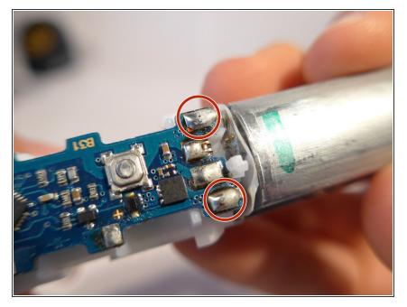
Now the connections to the motor have to be desoldered to take the battery casing of.
