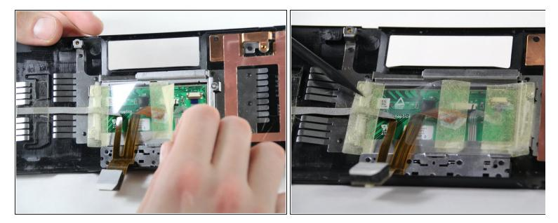
• Remove the tape, using the spudger if necessary.
