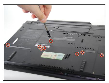
• Remove the eight 14mm screws using the Phillips #0 Screwdriver.
