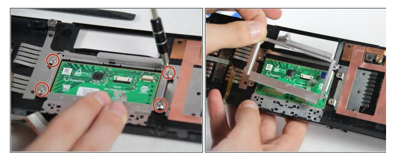
Use the Phillips #0 Screwdriver to remove the screws of the frame around the trackpad circuit board.
