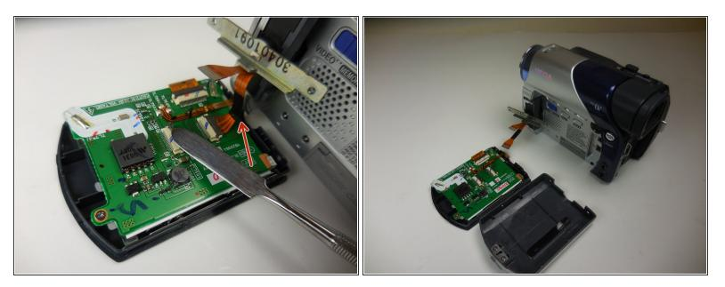
Carefully remove the wires connected to the screen from the black box. Now you will be able to separate the screen from the camera.
