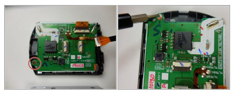
Unscrew the 5 mm Phillips #0 screw that is connecting the screen to the plastic casing.
