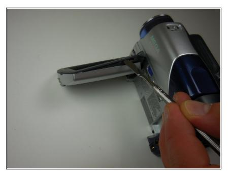
Pry apart the plastic casing around the screen using a flat spudger tool
