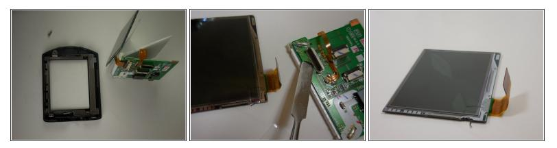
• You can now take out the screen to be replaced. Carefully remove cables from the data board.
