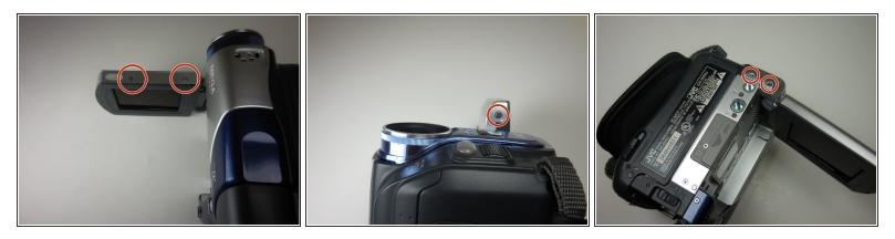
Unscrew 3 mm Phillips #0 screws around the LCD Screen. You will have to turn the screen to get the screws on the bottom of the screen.
