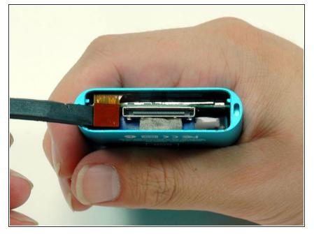
Use a spudger or the tip of your finger to carefully disconect the orange click wheel ribbon from the logic board.
