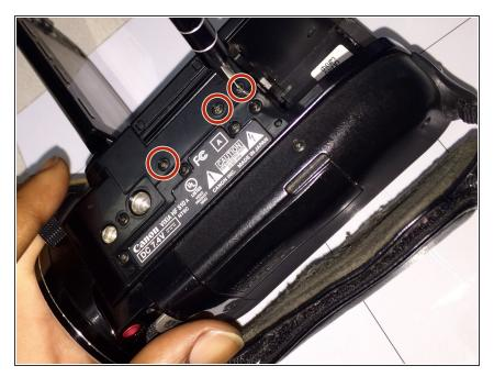
• Flip the camcorder upside down and remove the three 3x4 mm Phillips screws highlighted in the diagram.
