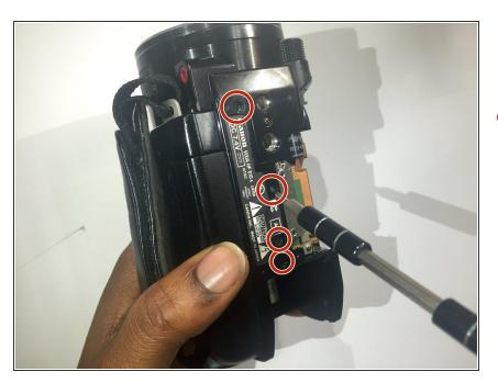
Turn the camcorder back to step one position and remove remaining screws on the bottom platform. There will be four 2x2.5 mm Phillips screws.
