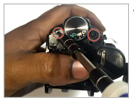
Remove the two 3x4 mm Phillips screws located under the coverings labeled AV & DCIN. These covers can be found when the back of the camera is facing you.
