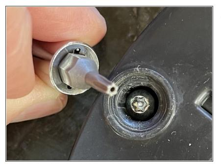
Also the front two screws are safety screws: they have a 6 sided star shape with a raised dimple in the center to prevent homebodies from casually opening the machine.
