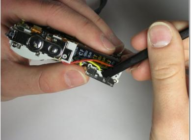
• Use the spudger to gently pry the top of the thin metal casing around the flash loose.
