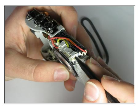
Pull the flash-bulb sub-assembly out of its place by using the pointed end of the spudger.
