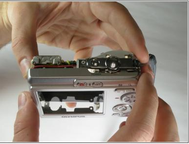
Ensure that the panels have been loosened. Carefully use hands to pull back and remove the panels.
