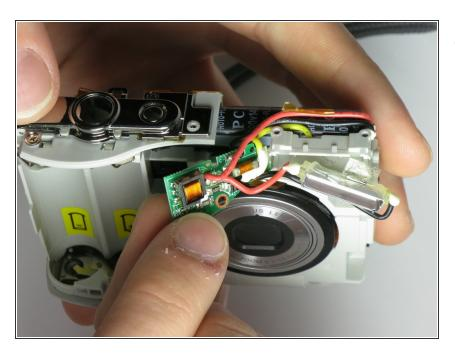
Pull the flash circuit board and flashbulb sub-assembly off from the front of the camera.
