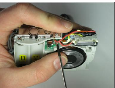
Remove the screw holding the flash circuit board in place.
