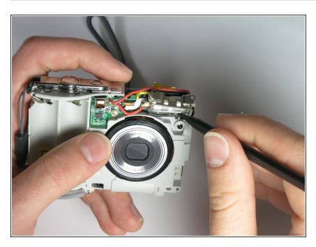
Use the spudger to gently pry the bottom of the thin metal casing around the flash loose.
