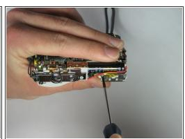
Remove the two small screws on the top of the flash itself.
