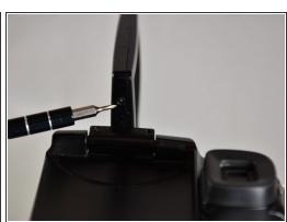
Unscrew the two 3 mm screws shown on the right side of the LCD screen panel.
