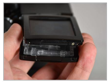
Pull off the back panel of the LCD screen and the plastic wire protector. Then replace the back panel.
