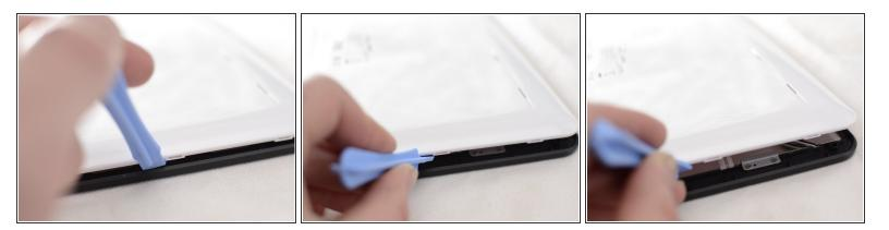
• Pry along the edge of the device to separate the back cover from the device.
