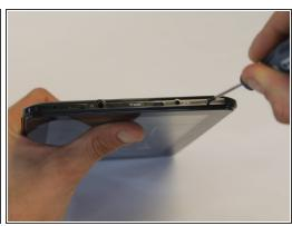
To begin, locate the two 4.9mm Phillips #00 screws at the top corners of the case and remove them.
