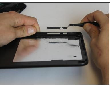
Carefully place the bottom lid next to the screen case. The power/speaker buttons should be visible at the corner of the lid. Remove the buttons with the tweezers.
