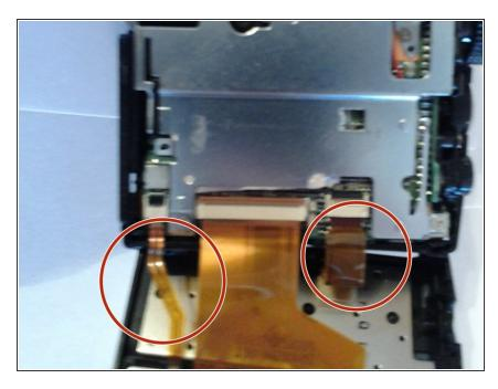
Once the back is removed, Do Not remove the ribbon cables shown in the within the red circles on the image.
