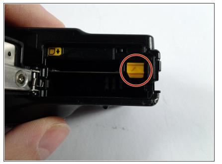
The SD card will be the smaller of the two cards in the battery terminal. Press down on the SD card and it will pop out enough for you to grab it and remove it. Then put another SD card in its place.
