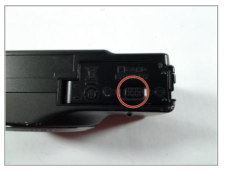
Start by locating the Battery Terminal on the bottom of the Camera, push the slider over to let the door flip open.
