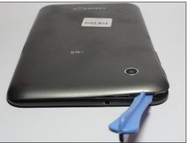
• Use the prying tool to separate the front and rear panels by slipping the tool underneath the screen edge and sliding it around the entire device.
