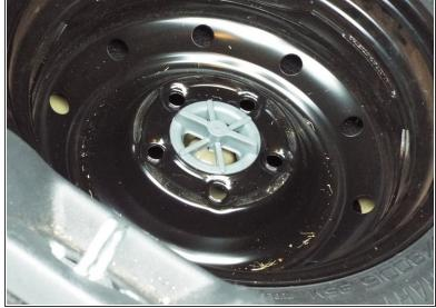
Turning counterclockwise, unscrew and remove plastic place holder in center of spare tire.
