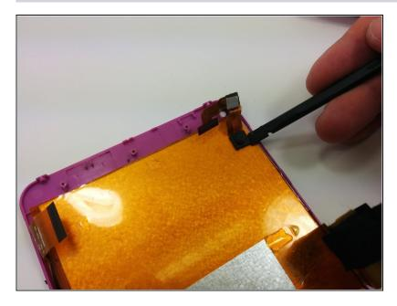
Using a spudger, gently pry off the camera from the back of the display
