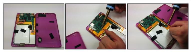
Use a soldering iron to remove the soldered connections on the motherboard
