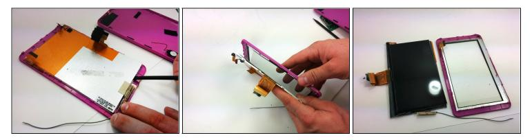
Using a spudger, separate the display surface from the front cover.
