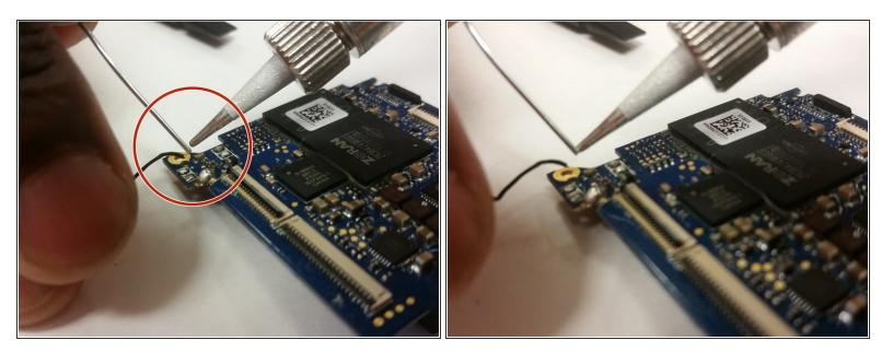
Last, solder on a functional motherboard at this stage and reassemble the device.
