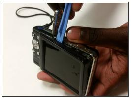
Use the Plastic Opening Tool and your finger to pry off and remove the external cover.
