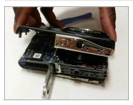
Remove the front cover of the camera using your fingers and the Plastic Opening Tool.
