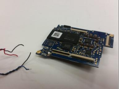
Desolder the four wires from the old motherboard.
