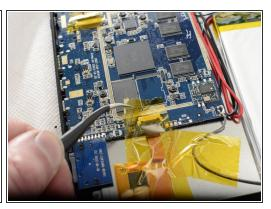
Remove the non-conductive tape located on the battery and motherboard assembly.
