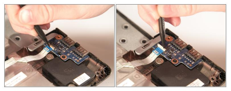
• Using a spudger, pry the ZIF connector upwards.
