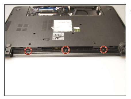
Remove three 2.9 mm Phillips #00 screws from the battery compartment.
