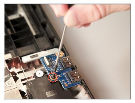
Using a #00 Phillips head screwdriver, remove the 2.9 mm screw on the USB circuit board.
