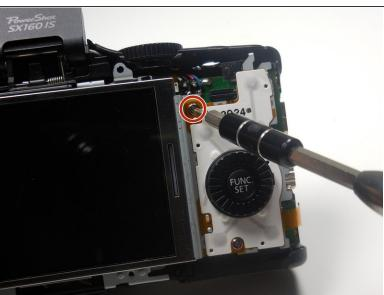
Use a #0 phillips screwdriver to unscrew the 3-3.75mm silver Phillips head screws from the function wheel panel of the camera.
