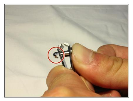
• Compress the body of the clippers to reveal the notch.
