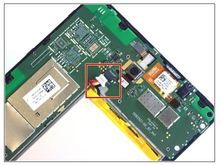
• Unclip the power clip from the motherboard by pulling down gently towards the bottom of the tablet.
