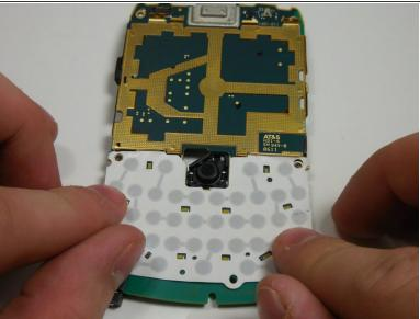
Align the new keyboard membrane with gold conduits and press down onto circuit board.
