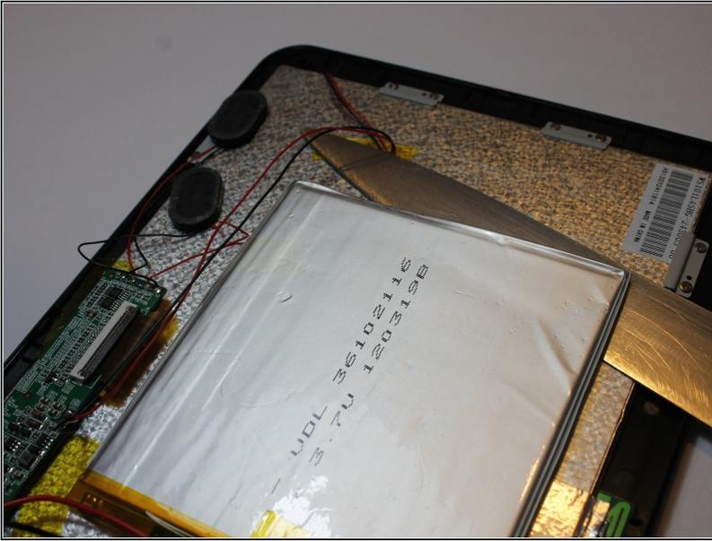
**⚠ WARNING:** Never use a knife or sharp object around a battery. Puncturing a battery may potentially cause a fire.
