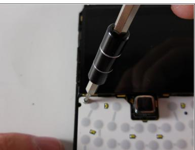
Remove the two Torx head 4.13mm steel screws with your T5 Torx screwdriver.
