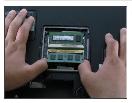
Carefully remove old/damaged RAM sticks and replace with new ones.
