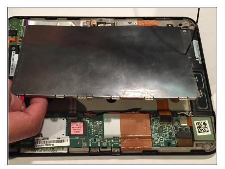
Lift the battery out of the device with your finger or the plastic opening tool.
