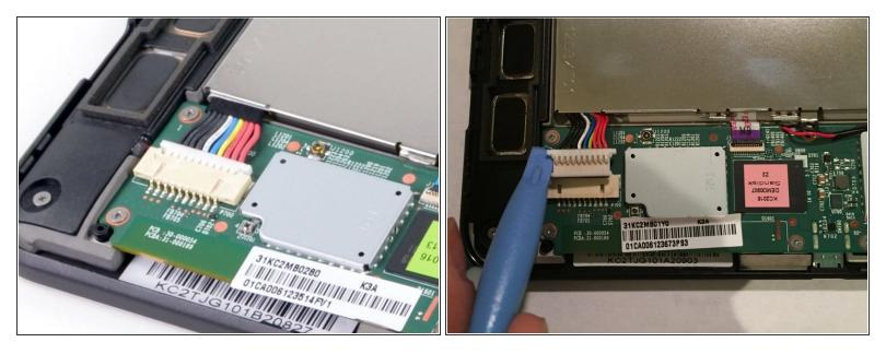
• Detach the plastic piece that connects the wires to the motherboard using the plastic opening tool.
