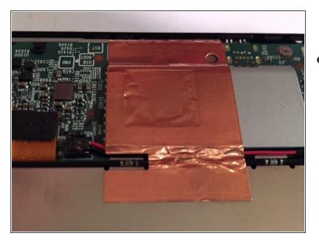
If your device has copper tape attached to the battery, carefully peel it off the battery.
