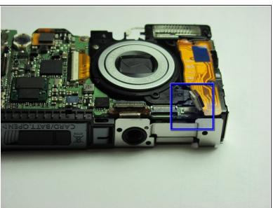
• Disconnect the connector at the bottom of the camera that attaches the flash to the motherboard by gripping it with you fingers and flipping it up.
