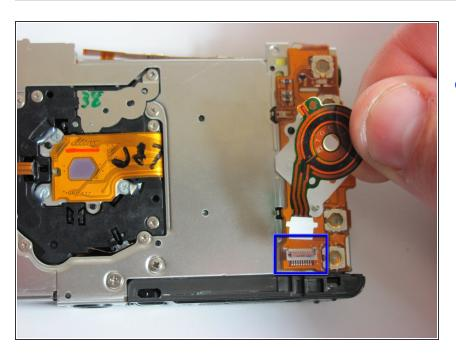
Disconnect the orange and black plastic ribbon that was underneath the circular rubber button by flipping up the ZIF connector and then sliding the ribbon out with your fingers.
