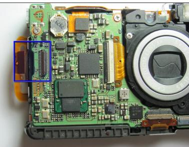
Disconnect the ribbon that attaches to the left side of the motherboard by flipping up the ZIF connector and then sliding the ribbon out.
