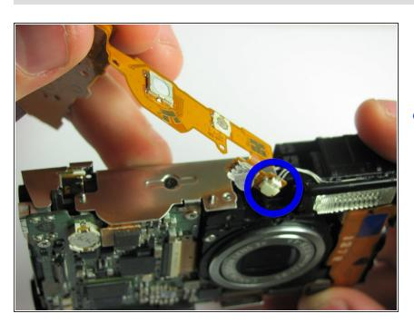
Disconnect the white connector on the top right side of the camera by pulling the wire out of the connector with your fingers.
