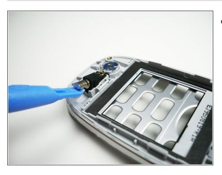
Use a plastic opening tool to lift the vibrator out of its slot.
