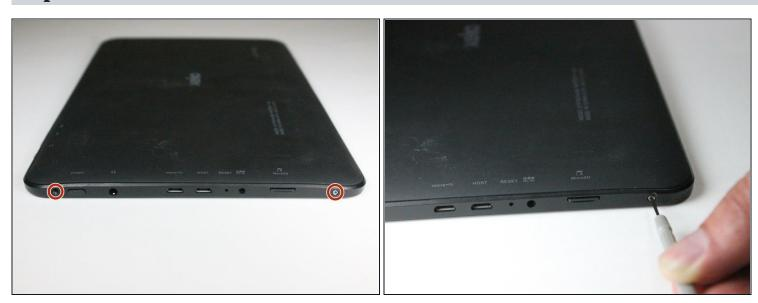
Remove the two 3 mm retaining screws from the side of the tablet with a Phillips #0 screwdriver.
