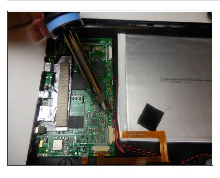
Use a soldering iron to remove the connection between the red wire first then proceed to the black wire. To reassemble your device, follow these instructions in reverse order.
