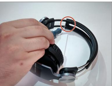
Remove the two 5mm Phillips #00 screws from each side of the headband connected to the metal track.
