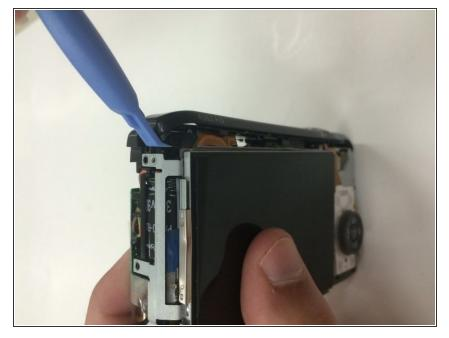
• After removing the interior left screws, use a plastic opening tool to gently pull the top face plate off.
