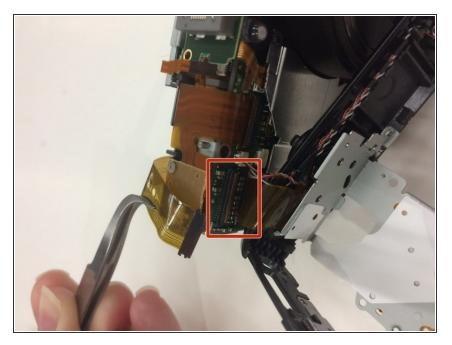
Carefully unplug the yellow ribbon cable from the front of the camera using your tweezers.
