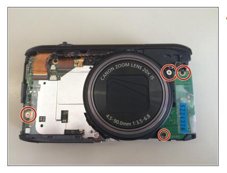
• Remove the 4 (3 mm) screws that are under the face plate.
