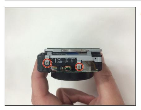
Next, remove the 2 (3 mm) interior screws on the left side of the camera.
