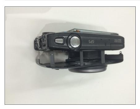
After removing exterior screws, gently lift off the front face plate with your fingers.
