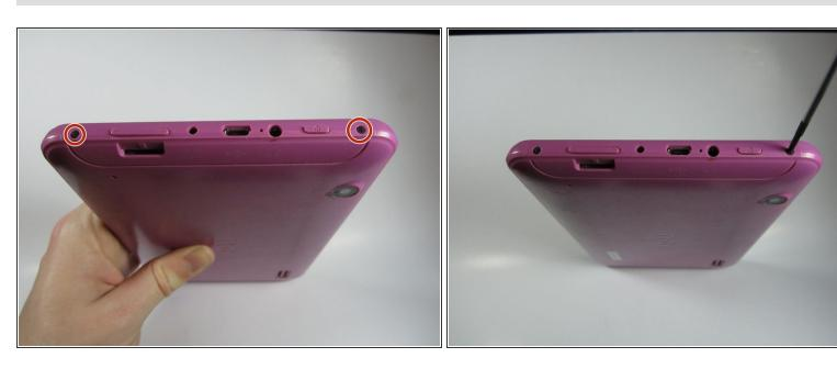
Use a Phillips #00 screwdriver to remove both 4.1 mm screws at the top of the device which hold it together.
