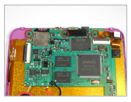
Use a philips #00 screwdriver to unscrew the three 4.064mm screws which attach the motherboard to the front of the device.
