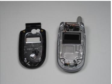
• With the edges separated, close the phone and lift off the faceplate with your fingers.
