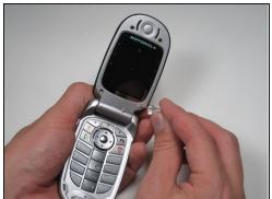
• Remove the four rubber stoppers from around the screen with a pin to reveal four screws.
