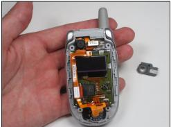
• Use a plastic opening tool to dislodge and remove the rubber camera cover.
