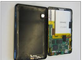
Remove back cover with plastic opening tool, exposing the battery and motherboard.
