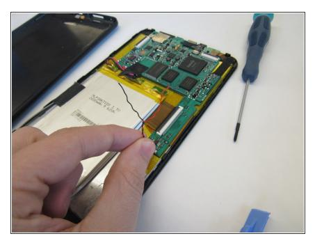
Uncoil the wires. If necessary, use a wire stripper to expose more of the wire.
