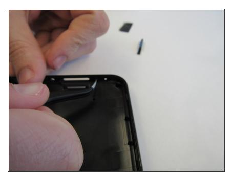
Dislodge the power button from the upper right corner of the tablet's back cover using the tweezers
