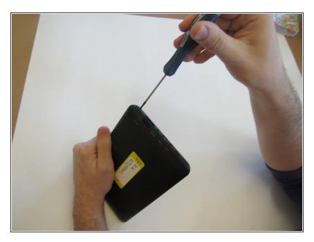
Remove the two 2.4mm x 4mm screws from the bottom of the tablet with a Phillips #00 Screwdriver.
