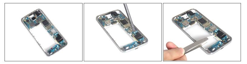
• Remove screw, release USB board flex connector and antenna cable connectors.
