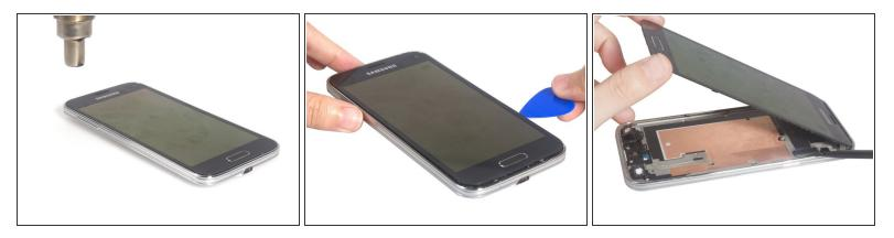
• Heat up the screen, cut the sticker and release the LCD screen connector carefully.
