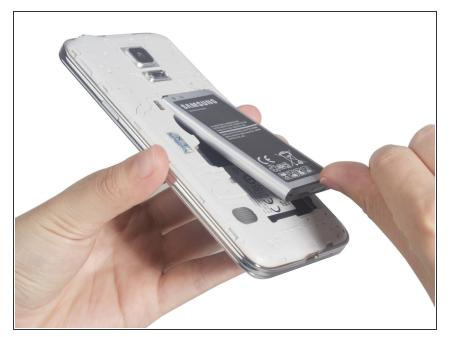
Remove battery. If you have the SIM card and SD card in, remove them by the way.
