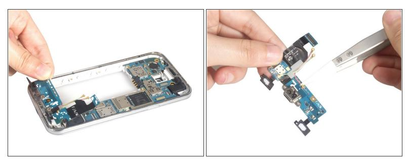
• Remove the daughterboard and clean the signal cables from assembly. And you can replace the new USB charging board for Samsung Galaxy S5 Mini.
