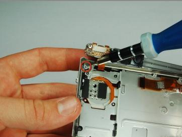
• Use a PH00 screwdriver to remove the 2.9 mm phillips screw on the upper left side of the case.
