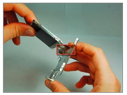
Pull the tape off that holds the LCD to the assembly.
