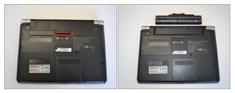
• Use a fingernail or plastic opening tool lift the battery while holding the release latch. Rotate the battery up and away from you to remove it from the laptop.
