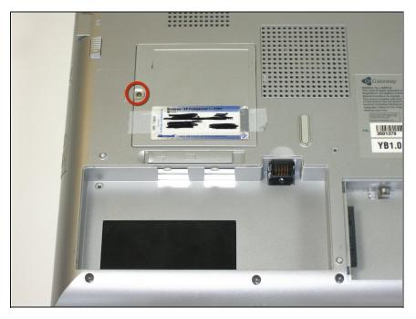
Remove access cover by unscrewing captive screw.
