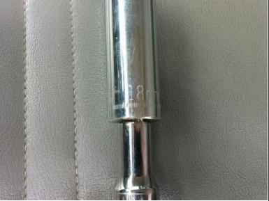
Adjust the seat as far back as you can. Using an 18mm deep wall socket, remove the bolts on the front that attachs the seat to the floor. On my bench seat there were only two bolts. If you have a 60/40 seat or bucket seats there will be more.
