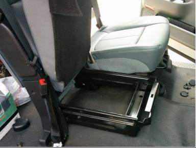
Next place your jump seat in the middle on top of the transmission tunnel. The rear holes will line up with two of the existing holes where the seat belts were attached. Place two bolts in the holes but don't tighten completely. Lift the bottom seat up exposing the two bolt holes in the bottom of the jump seat.
