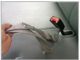
Using the T60 Torx bit, remove the bolts attaching the seat belt receivers to the floor and remove the seat belt receivers.
