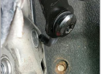
• In my case the seat belt buzzer on the new seat didn't match the vehicle plug. Simply remove the seat belt receiver from the side of the seat with a T60 Torq bit and re-attach your old seat belt receiver to the floor bolt. Using the old seat belt receiver gives you the proper connector and allows the buzzer to work properly.
