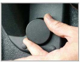
Place your bucket seats in the truck. You should be able to line up all 4 holes in the seat frame with a hole in the truck body. You may use the same bolts you removed from the old seat to bolt the new seats down. Replace the plastic bolt covers on the new bucket seats.
