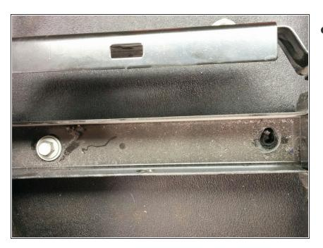
Now mark and drill two holes in the transmission tunnel. Carefully check what is below the tunnel to make sure you don't damage wiring or other system that may be run along the path. This is best done with one person drilling and one person watching underneath. These are the only holes you must drill for 2011 to 2014 seats to fit.
