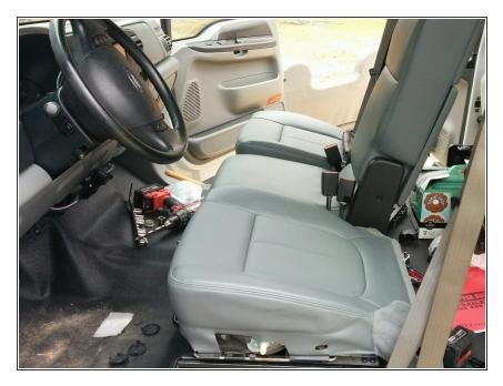
Notice the jump seat is a little lower than the buckets. Place your buckets in temporarily and use washers or other spacers between the floor and jump seat frame to adjust the jump seat to the same level as the buckets.
