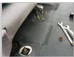
Adjust seat to it's most forward position. Look for a stud with a plastic protection cap. Remove the
