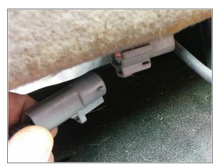
Unplug the seat belt receiver from the vehicle seat belt buzzer plug. it will be just under the back side of the seat.
