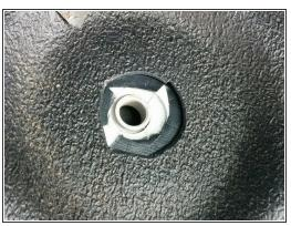
Next, if your truck was only using the outter body holes you will need to locate the two close to the transmission tunnel. You can press your finger in the center and locate the opening. Take a razor knife and gently cut an X over the hole. Gently remove each of the triangle shaped tabs exposing the additional hole. Repeat on opposite side.
