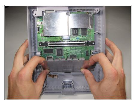
• Lift the front shield straight up to remove it from the motherboard.
