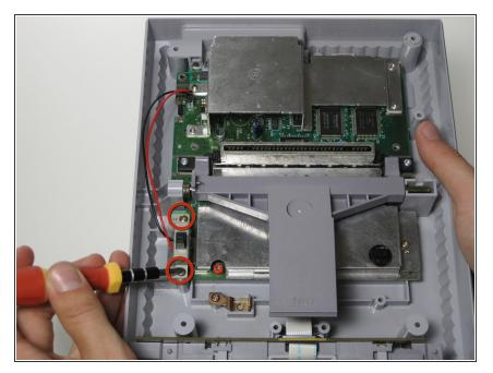
Remove the two 11.7 mm Phillips #2 screws connecting the power switch to the motherboard.
