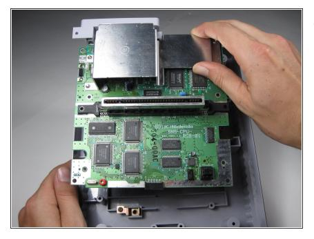
• Lift the motherboard straight up to remove it.
