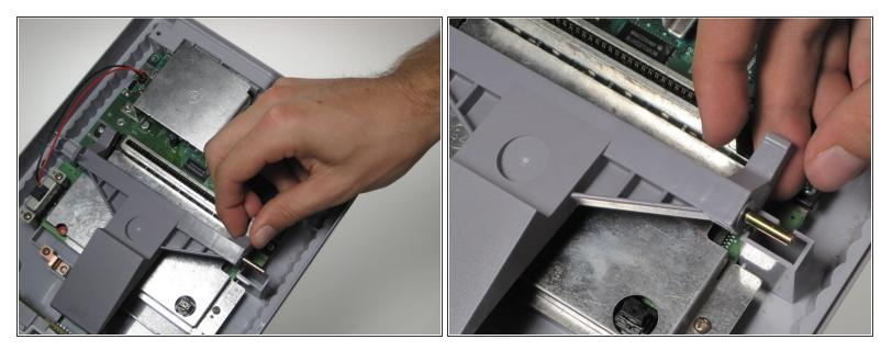
• Lift the right side of the eject lever out of the housing.
